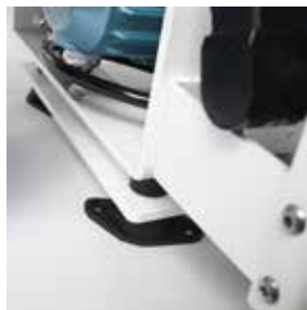
Vibration-isolation mounts reduce noise and vibration.
